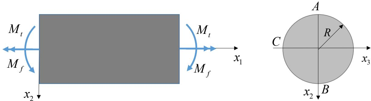
Determine the components of the deviatoric stress tensor  $s_{ij}$  and the effective stress  $\sigma_e$  at points  $A$ ,  $B$  and  $C$ . Comment on the results. Note that the stresses due to bending and torque are given by  $\sigma = M_f x_2 / I$ ;  $\tau = M_t r / I_p$  with  $I, I_p$  indicating the moments of inertia around the bending axis and the polar moment of inertia, respectively. For a circular cross-section we have,  $I_p = 2I = \pi R^4 / 2$ .
